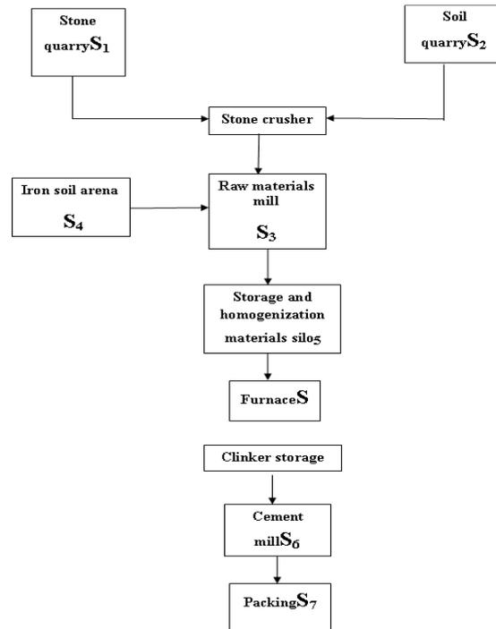
Figure 8: The Suggest Test Point in Technical Route of Al Muthanna Cement Plant
