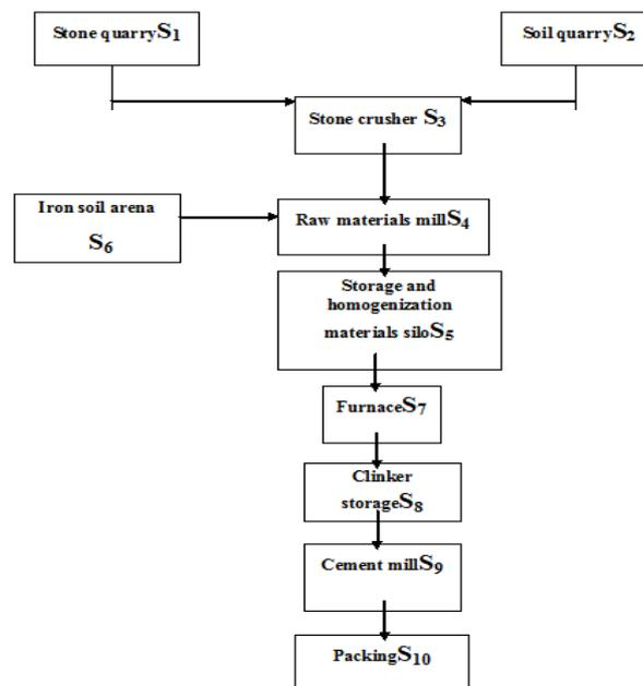
**Figure 1: Test Point in Technical Route of Al Muthanna Cement Plant**
